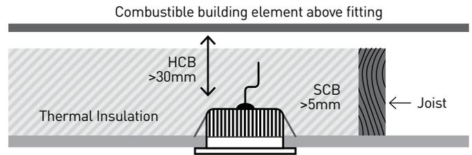
Note: Not Suitable for use with loose-fill insulation.
