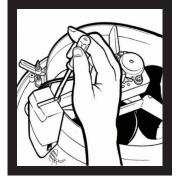
4. Remove terminal cover and wire according to the diagram in Option 1 over. This method of wiring switches fan and light on and off simultaneously. Option 2 shows how to wire fan and light separately. This allows the light (or the fan) to be switched on independently of the other. Option 3 shows the addition of a HPM Cat TX770/1RC time delay mechanism.
