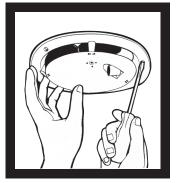
Turn the retention screws clockwise. The toggles will splay out. Tightening the retention screws allows the toggles to grip the ceiling material.
