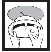
5. Remove light diffuser and air-intake grille. Unscrew the 3 screws on the lip of the unit until the gap between the toggles and inner lip of the unit is greater than the width of the Gyprock, or other ceiling material. Fold these toggles in. Push unit into hole.
