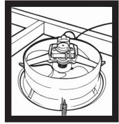
It is recommended that the three toggles be checked for the correct clamping by inspection from above.
