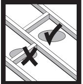
Determine position in ceiling where Fanlight is required to be installed. (Do not install within 120cm of stove or inside a shower recess). Be certain that the installation area is not restricted by roof beams above
