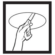
3. Use electric jig saw or small hand saw to cut out around this line. Several holes drilled at a point inside the circle provides a convenient starting point for cutting the panel out.
