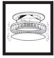
You may now insert a globe (not more than 75W) into the lampholder. Push grille into unit and click into position. Assemble the diffuser and round dust seal and twist into position. To remove this assembly for cleaning, simply pull assembly downwards. For globe changing only, simply twist the diffuser anticlockwise and remove.
