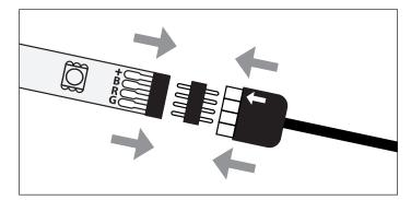
Connect the driver to the powerpoint and switch on. Check that all LED strips are working. If this is not the case, switch off and adjust the connectors.
