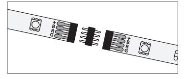
**To shorten the strip:** scissor markings allow cutting of the strip every 100mm. **Important:** Once a strip is cut, it cannot be connected to another strip. Only the last strip can be cut.
