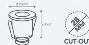
\* The 15W LED driver (supplied with LDR01DECK) can take a maximum of 25 deck lights (LEDK013K316)
