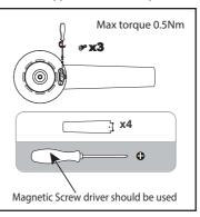
B. Assemble the cover plate to the motor housing with 2 x screws provided. Max. torque to 0.5 Nm.
