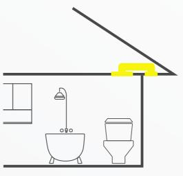
**1. CEILING MOUNTED FAN** Designed for low-pitch roofs or between floors, where there is no ceiling access. Also available
