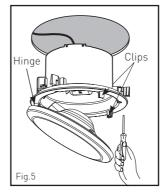
5. Unclip 2 x reflector clips and
