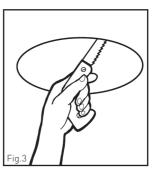
3. Use an electric jig saw or small hand saw to cut out around this line. Several holes drilled at a point inside the circle provides a convenient starting point for cutting the panel out.
