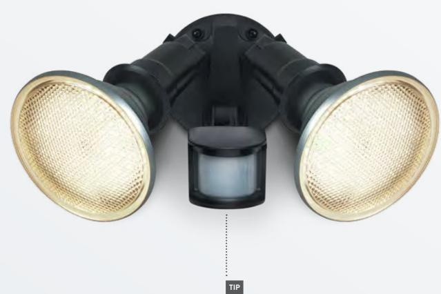
Passive infrared sensors are sensitive to a person's skin temperature through emitted body radiation, in contrast to background objects at room temperature. No energy is emitted from the sensor, thus the name "Passive Infrared" [PIR]
