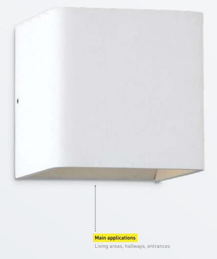
8.3W Power Lumen output Warm White 335 lm 40 lm/W Efficacy Warm White Colour temperature Warm White 3,000K 80+ CRI Lifespan 30,000 h Construction Electroplate with white finish 8.3W LED up/down light fixture, Package contents wall plugs and screws Product code White Finish Warm White Light LWL053KWE
